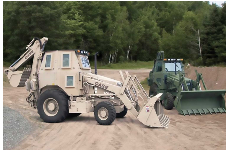
The High Mobility Engineer Excavator Type I (HMEE-I) is a non developmental military vehicle fielded to the Army's Brigade Combat Teams (BCT) and other selected engineering units. Tasks performed by the HMEE-I and III include repair and improvement of roads, trails, bridges and airfields.
