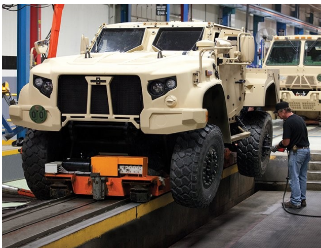
Contractor installs tires on the Joint Light Tactical Vehicle production line in Oshkosh, WI
