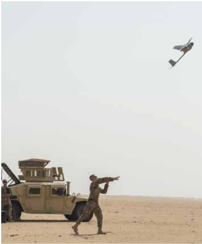
A soldier with the 197th Field Artillery Regiment throws an RQ-11 Raven unmanned aircraft system at the start of a flight mission at Camp Buehring, Kuwait.
