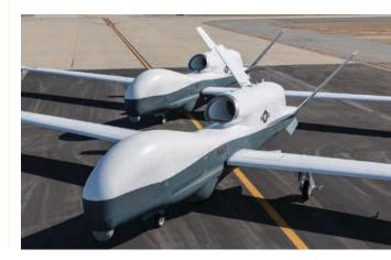
persistent-sensor dwell and ability to network its data, deliver a capability that will enable the MPRF family of systems to meet the Navy's maritime ISR requirements. A single *Triton* orbit provides continuous surveillance capability at a maximum mission radius of 2,000 nautical miles for a minimum of 24 hours. At full operational capability, the system will provide up to five simultaneous orbits worldwide.
