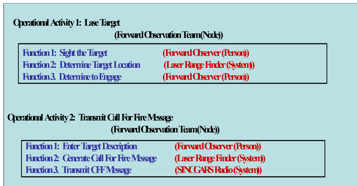
Figure 2-6: Relating Functions to Systems, Applications, and Personnel
