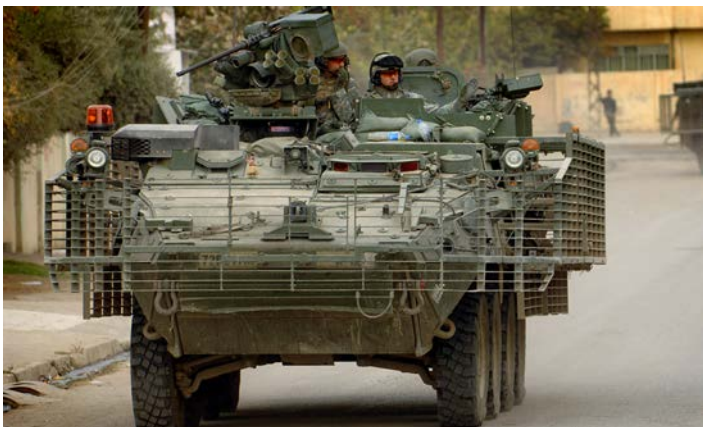
This Stryker, on patrol, is an eight-wheeled, all-wheel-drive, armored combat vehicle. This vehicle is part of the Army's Combat Platform modernization.
