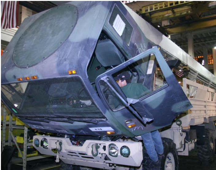
An M1078 Lightweight Medium Tactical Vehicle goes through Reset at the Red River Army Depot in Texas.
