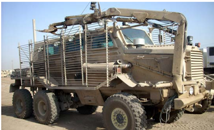
A Buffalo Mine Protected Clearance Vehicle provides a blast resistant platform to protect Soldiers and their equipment during mine clearing operations.
