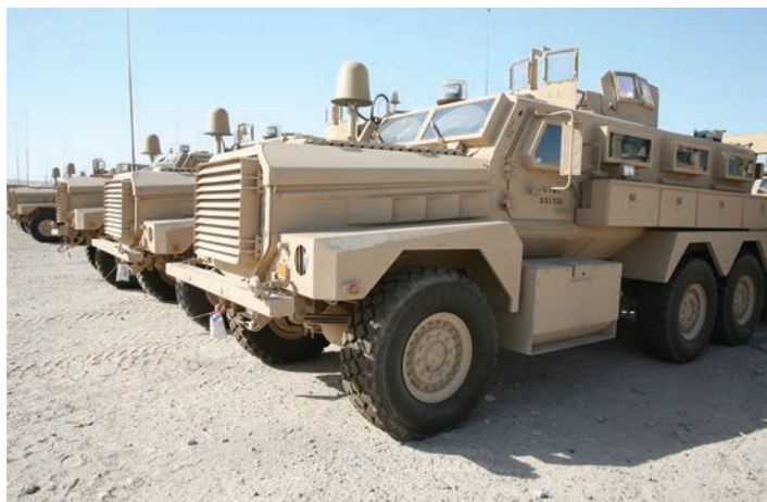
These Mine Resistant Ambush Protected vehicles are armored vehicles designed to survive Improvised Explosive Device attacks and ambushes.
