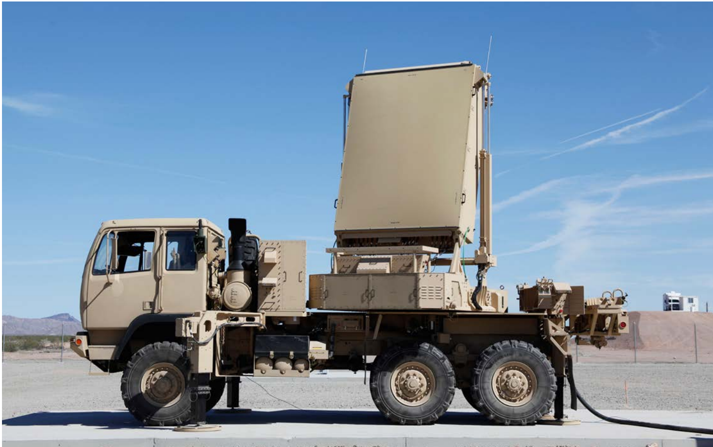
EQ-36 Counter Fire Radar is designed to locate the firing positions of both rocket and mortar launchers.
