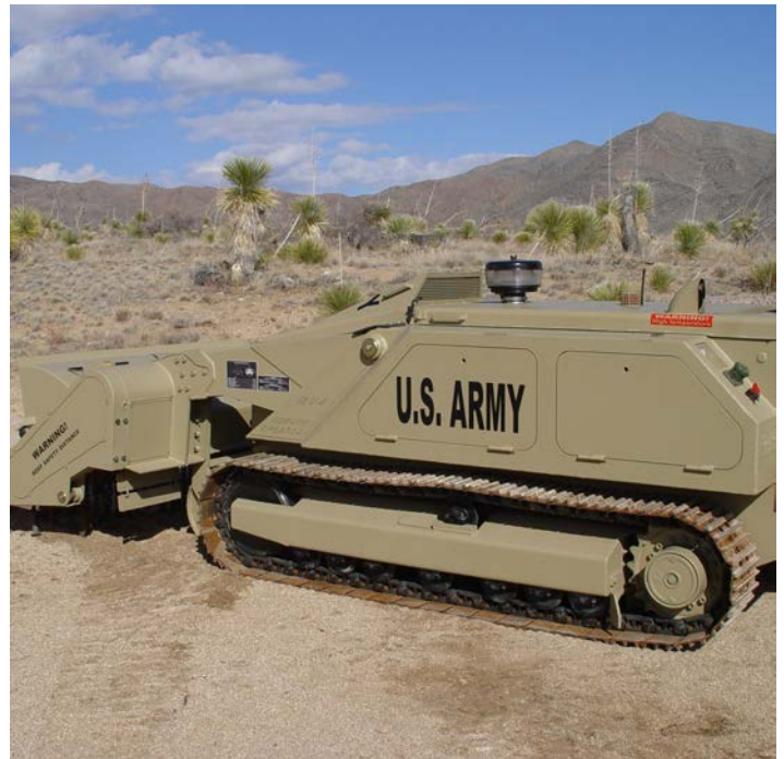
The unmaned MV-4 Mini Flail is designed to clear various types of terrain containing anti-personnel mines.
