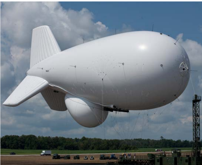
The Joint Land Attack Cruise Missile Elevated Netted Sensor (JLENS) protects our Soldiers over a large area by providing over-the-horizon surveillance for defense against cruise missiles.
