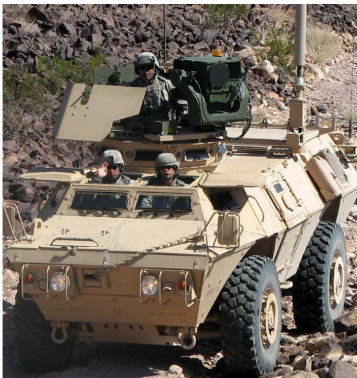
The M1200 Armored Knight is designed to provide precision strike capability by locating and designating targets for both laser-guided and conventional munitions.
