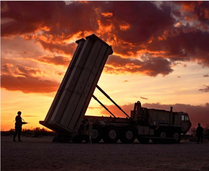
The Terminal High Altitude Air Defense (THAAD) formerly called the Theater High Altitude Air Defense is designed to shoot down short- and medium-range ballistic missiles using a hit-to-kill approach.
