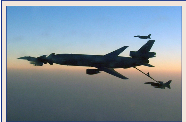
A KC-10 Extender from the 908th Expeditionary Air Refueling Squadron refuels F-16 Fighting Falcons Feb. 1, 2010, over Afghanistan, during Operation Enduring Freedom air refueling operations. (U.S. Air Force photo by Capt. Sean Chuplis)
