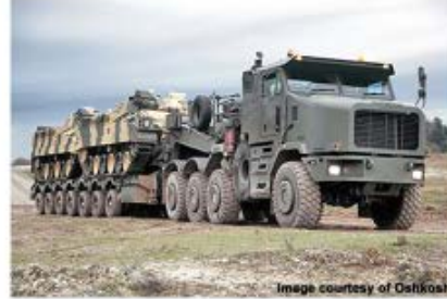
Heavy Equipment Transporter (HET)
