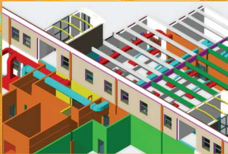
BIM Benefits: Faster Delivery, Better Quality, Less Expensive. BIM allows engineering analysis and interference checking between disciplines, reducing change orders and improving design decisions. (BIM of Army Reserve Center, courtesy Louisville District BIM Team)
