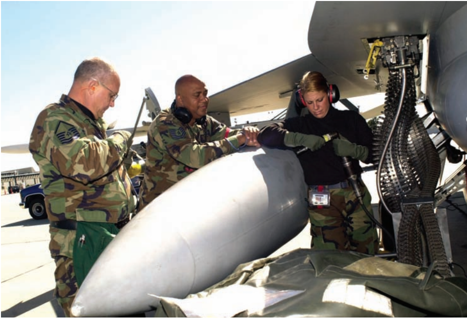
Master Sergeant Franklin Buzby (left), Technical Sergeant Wendell Hunte (center) and Senior Airman Tina Ghaffins (right) from the Aircraft Generation Squadron, 177th Fighter Wing, New Jersey Air National Guard, use a Universal Ammunition Loader to load 20mm rounds used in the F-16C Block 25. The Wing was flying combat air patrol missions during Operation Noble Eagle. (Photographer: MSgt Tom Louis. Courtesy of 177th Fighter Wing.)
