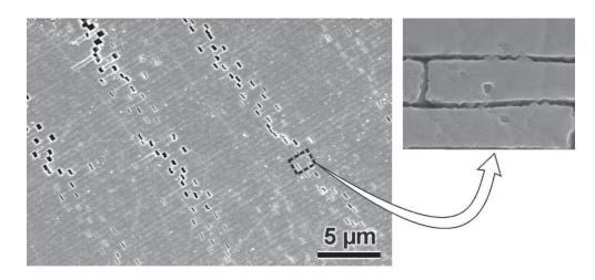
FIGURE 5-4 Structure of an abalone shell.
