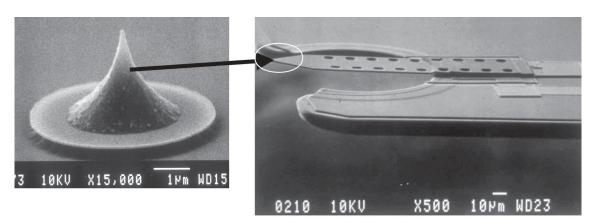
FIGURE 6-2 A micromachined cantilever and tip-mounted stylus designed for readout using a separately positioned fiber-optic reference. Source: Reprinted with permission from Kong et al., 1993. Copyright 1993, Journal of Vacuum Science and Technology.
