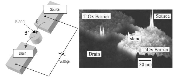
FIGURE 6-4 Schematic drawing and structure of a single-electron transistor for measuring electronic charge. Source: Quate, 2000.
