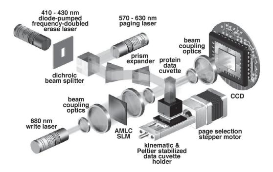
FIGURE 4-2 Schematic diagram of a protein-based, 3-D memory capable of storing between 7 and 10 gigabytes of digital, error-corrected data in a rugged  $1 \times 1 \times 3$  cm<sup>3</sup> polymer cuvette. These inexpensive cuvettes can withstand virtually any condition that a human can withstand, including submersion in water for extended periods of time. Selected components are labeled as follows: AMLC SLM = active matrix liquid crystal spatial light modulator; CCD = charge-coupled device.
