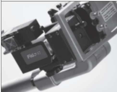
The Fido XT provides a wide-view camera and an explosives sensor on its highly maneuverable and extendable arm. It is ideal for "sniffing" out explosives from under vehicle chassis, car trunks and inside vehicles. Soldiers can operate the device from a safe distance. (U.S. Army photo.)
