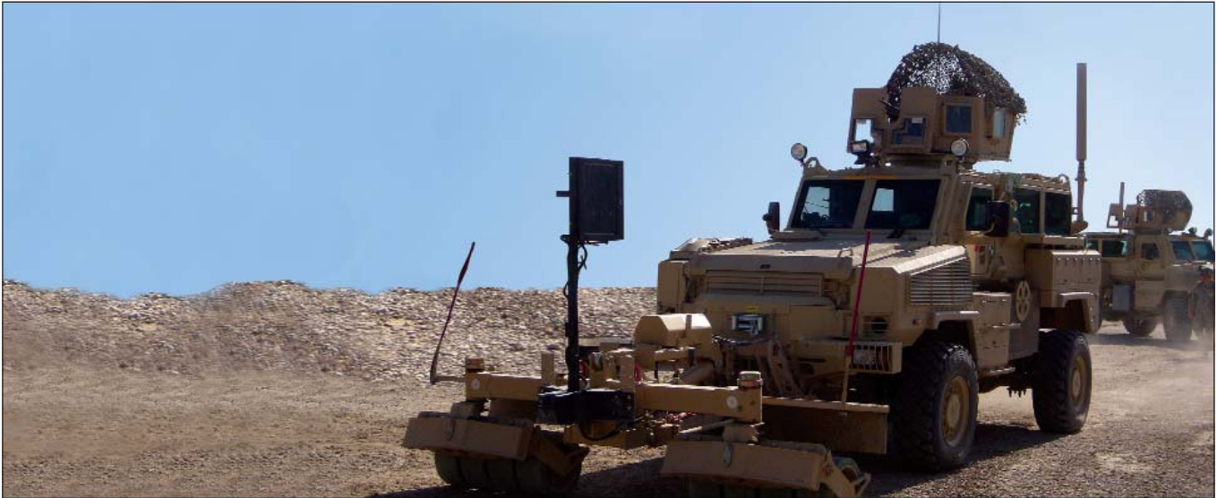
Project Manager (PM) Close Combat Systems/PM Improvised Explosive Device (IED) Defeat has fielded more than 360 SPARKs to Soldiers in the GWOT. The SPARK provides additional stand-off capability to vehicles and crews against pressure-activated IEDs. (U.S. Army photo courtesy of TARDEC.)
