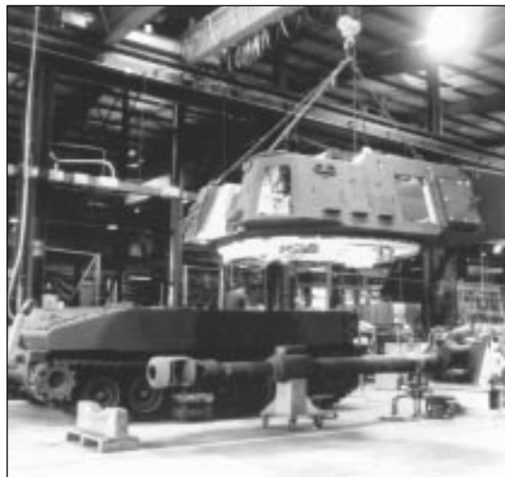
New larger cab being joined to completely refurbished chassis at Letterkenny Army Depot.
