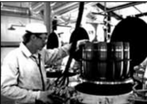
Autoclave Meltout: An autoclave operator lowers projectiles into a pressure vessel where steam will melt out explosives that can be reclaimed.
