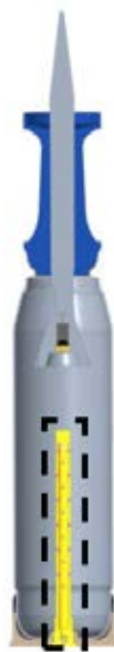
The first 120 mm cartridges qualified with the M125 thin-walled body primer in 1984. (Image courtesy of the author)
