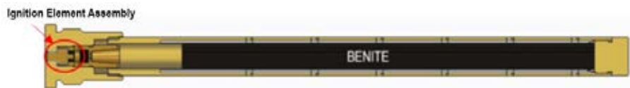
The ignition element assembly in the M125 electric primer hadn't changed for almost 40 years. (Image courtesy of the author)
