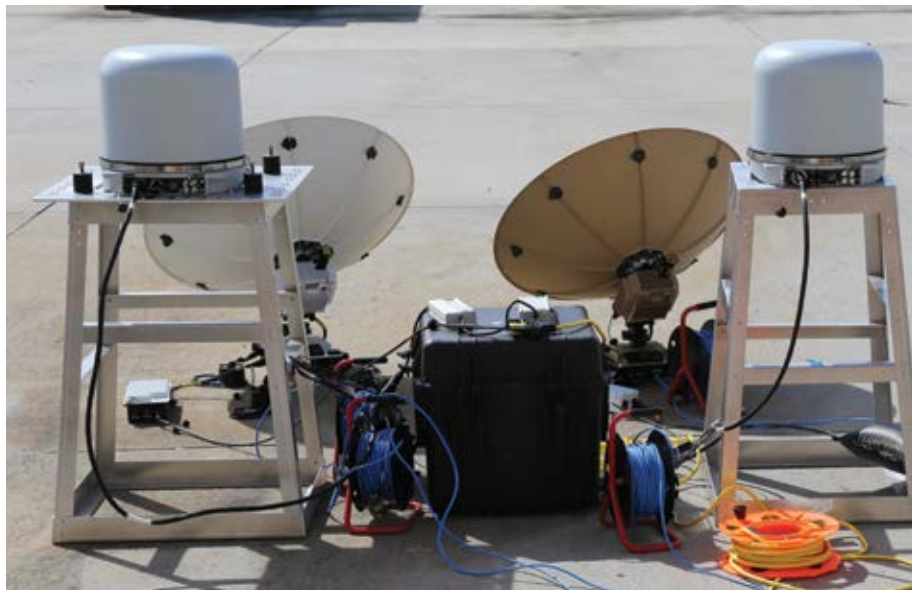
Industry-provided MEO and GEO ground satellite prototype terminals are seen here during an early Army assessment of managed multi-orbit satellite communications capabilities and services, in March at the Joint SATCOM Engineering Center, at Aberdeen Proving Ground, Maryland. (Photo by Amy Walker, PEO C3T)
