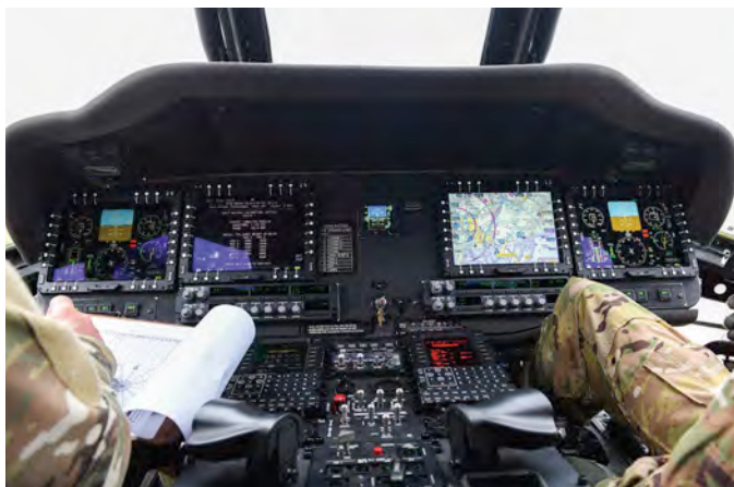
After: The digital cockpit of a UH-60V.
