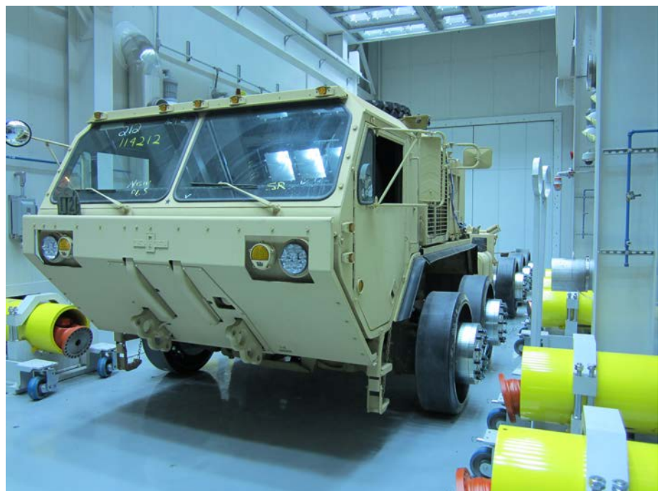
The Palletized Loading System (M1074A1) in PEVEL for mobility performance testing at 120 degrees. Using the “oven” for actual ambient temperatures produces much more accurate results. (Photo by Stephen Roberts, GVSC)
