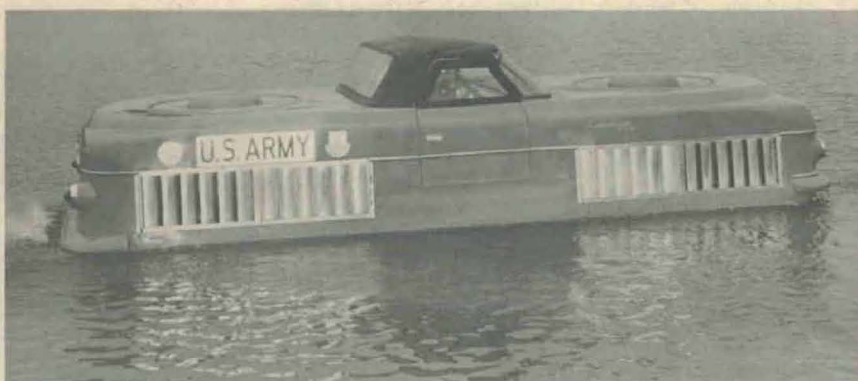
GEM (Ground Effects Machine) craft promises speedy, economical amphibian transportation in future. Air jets lift it above surface for forward progress.
