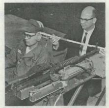
David Penneman, HEL engineer, takes measurement between subject and M6-machinegun during demonstration of a system he helped design by which hearing tolerance to impulse noise can be reliably determined. shows that less than eight percent of the total Army strength requires the lighter equipment. Current standard items could continue to be issued to all other soldiers with missions less demanding in terms of close enemy contact.
