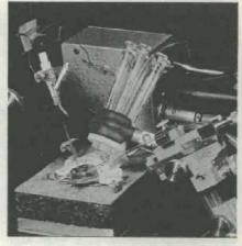
IN OLFACTORY NERVE CODING study in frog, microelectrode (left) is connected to preamplifier. Glass tube (right) passes air through nostril to supplant natural breathing. Various odors are introduced with syringe assembly (center) and patterns of nerve pulse activity are observed on oscilloscope (not shown).
