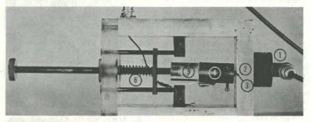
EXPERIMENTAL ARRANGEMENT for studying semiconductor transducer performance. A conventional transducer (1) transmits a pulse of ultrasonic energy through an aluminum plate (2) where it is picked up by the semiconductor crystal (3) mounted in a metal holder (4). A piece of lucite (5) isolates the holder from the spring mechanism (6).
