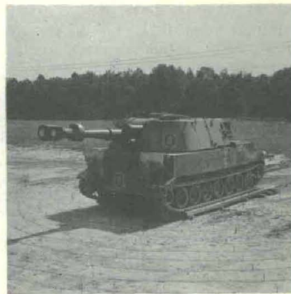
RINGS OF RADIATION surround M109 self-propelled howitzer at NDL test area where scientists simulate atomic exposure by passing radioactive source through plastic tubes arranged in circles around test subject.
