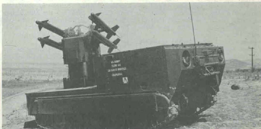
ARMY DEVELOPMENT OF CHAPARRAL, a new air defense guided missile system designed to combat low-altitude attack, advanced early in October with a successful firing at China Lake, Calif., Naval Ordnance Test Station. Chaparral uses a modified self-propelled vehicle (XM548) as a mount for launching the heat-seeking Sidewinder missile. The Sidewinder, originally developed by the Navy as an air-to-air weapon, has been modified slightly for Army use.
