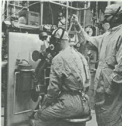
AEROSOL GENERATING equipment at Army Medical Unit at Fort Detrick, Md., can be adapted easily for exposure of humans or animals to precisely measured quantities of biological products for research experiments.
