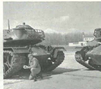
T142 RETREADABLE tracks are shown on the tank at left. The entire standard T97E2 track (right) must be replaced when excessively worn.
