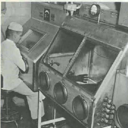
SEALED MICROTOME unit coupled to a biological safety cabinet is employed at the U.S. Army Medical Unit to provide safety for personnel preparing frozen sections of infected tissues for microscopic examination.
