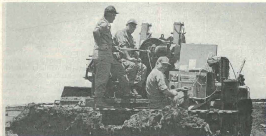
ON LOCATION in Central Highlands of South Vietnam, Henry Wysocki (center) and Stephen Doherty (right), AMMRC, operate Magnetic Recording Borescope in field tests to evaluate more accurately the service life of 175mm gun tubes.
