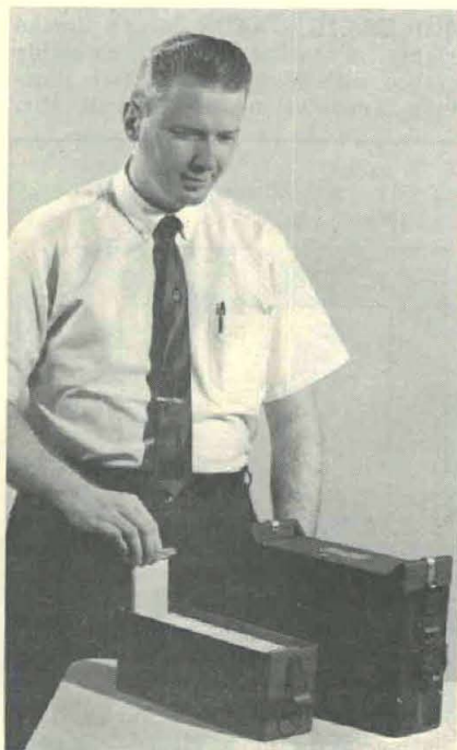
TWO SIZES of basic cell of Army's mechanically rechargeable zinc-air battery are shown above. Cigar pack is for size comparison. At left, David Sague, ECOM electronics engineer, inserts a zinc anode into 20-ampere version of zinc-air battery for field use. The battery in the background has a 48-ampere hour capacity. Both are in the 12 to 24-volt operational range.
