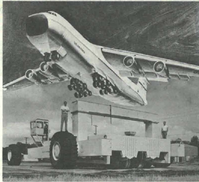
TEST LOAD CART is used at Waterways Experiment Station to obtain data for designing efficient landing gear. Two load carts, each mounted on six wheels, are designed to simulate undercarriage of C5A aircraft shown above.
