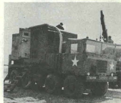
PERSHING Power Unit, mounted on new 8-wheel, 5-ton cargo truck, consists of the Improved Programer Test Station and Power Station. Both pairs of front wheels are steerable for substantially increased maneuverability.
