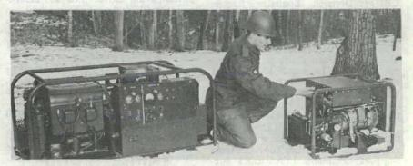
FAMILY OF TURBO-ALTERNATORS is being developed at MERDC to cut costs and ease logistical problems involved in generating electric power in the field. The 10-kw unit shown here is one-fifth as big and weighs 725 pounds less than the standard Army 10-kw engine generator it is designed to replace.
