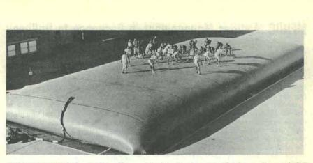
STORAGE TANK for 27,000 gallons of fuel is displayed in the form of one of the world's most unusual gridirons. Made of nylon coated with polyurethane, it is the largest of a family of self-supporting "pillow" tanks developed to provide mobile combat forces with unit that can be quickly erected and disassembled.
