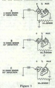
from zero to 15 ohms (Figure 1B), the current divides after passing through the left coil. One-third of the current passes through the 30-ohm-resistance right coil to ground; and two-thirds passes through the 15-ohm sensor to ground.
