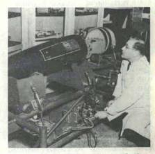
Abraham Grinoch, chief of the Evaluation Branch, Technical Services Directorate, prepares a nuclear missile warhead section for testing in the radio-frequency hazard simulation chamber, new Picatinny Arsenal facility.
