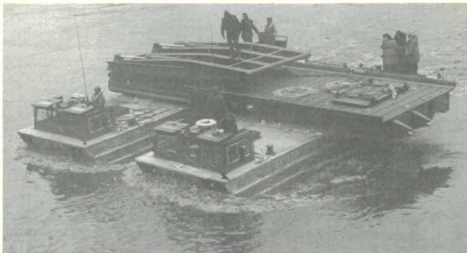
PREPRODUCTION MODELS of the Mobile Assault Bridge/Ferry (MABF), developed by the U.S. Army Mobility Equipment R&D Center, Fort Belvoir, Va., are shown here undergoing tests on the Mohawk River at Schenectady, N.Y., near the Consolidated Diesel Electric Co., where they were built. The two units shown are an end bay and an interior ramp coupled to form a 2-bay raft. A multiyear, multimillion dollar contract will provide 122 units with interior-bay and 62 with end-ramp superstructures.
