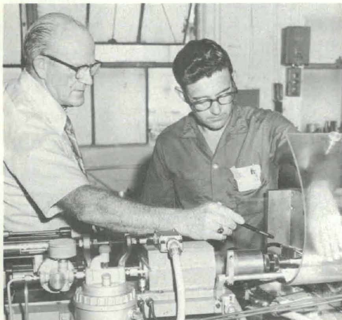
PICATINNY ARSENAL production engineer Robert Findlay and Roderick Muck, a machine tool job setter, check copper cone during machining process developed to meet critical tolerances in arsenal's production of shaped-charge ammunition liners.
