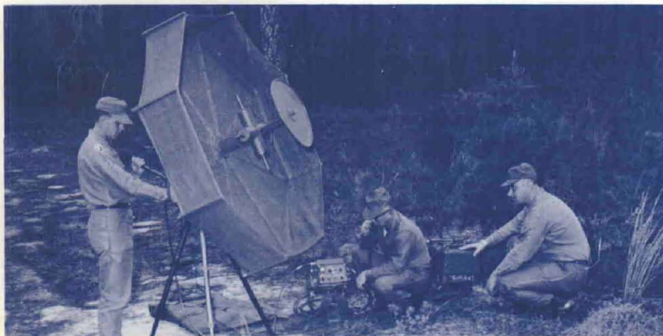
UHF tactical satellite communications team-pack terminal linked troops of the 75th Arctic Rangers on icecap with the Alaskan mainland in Exercise Ace Band Polar Cap II.
