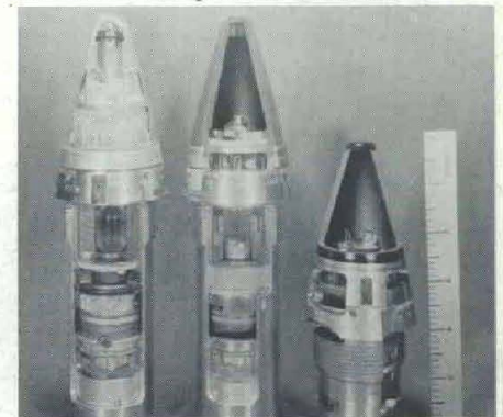
PROXIMITY FUZES for artillery-caliber shells (from left) include the first fuze developed by the Navy during the Korean Era, HDL's product-improved fuze, and the latest, which uses integrated circuits.
