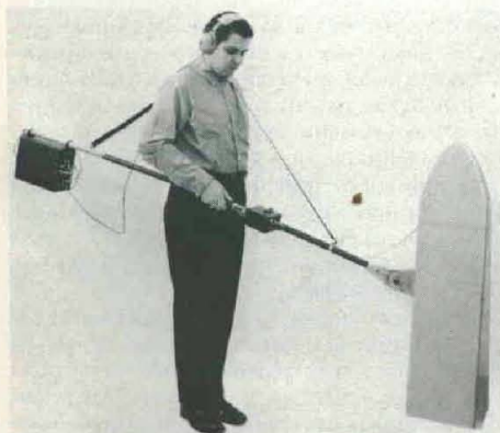
PORTABLE RADAR , developed to detect mines and other subsurface explosives, is being tested to locate buried objects such as utility conduits, human bodies.
