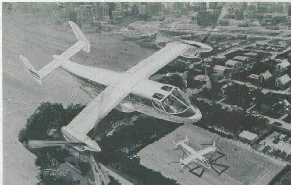
XV-15 V/STOL tilt-rotor research aircraft. The Bell Helicopter Co. will design, manufacture and test two prototypes in a program sponsored by the Army and NASA.
