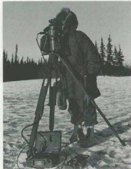
SSG Michael Garcia, Fort Leonard Wood, MO, takes a bearing with a new lightweight azimuth gyro surveying instrument during its winter evaluation at ATC.
