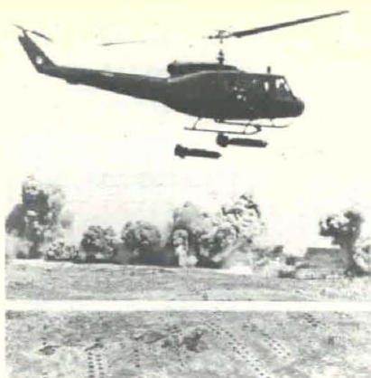
Fig. 4. FAESHED Mine Neutralizer, consisting of two Navy CBU-55/B weapons mounted on an Army UH-1H helicopter, breaches a live minefield.
