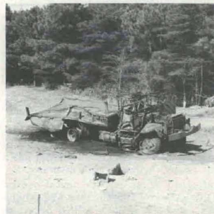
Fig. 3. FAE blast effects on 2½-ton cargo truck would have been fatal to personnel in the truck as well as in two nearby foxholes where wooden targets were shattered during tests.
