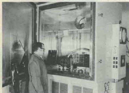
RUBBER-COATED FABRICS Research Group's Paul Touchet checks items for text in a cold box used in low-temperature research to develop ozone-resistant rubber.
