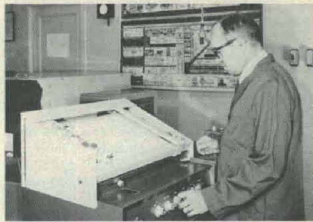
RADIATION RESEARCH Group's Ed Heck works with Ratio Recording Spectrometer to measure transference and reflectance properties of liquid and solid materials.
