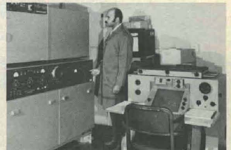
CHEMISTRY BIODETERIORATION Group's Frank Harris works with a Direct Reading 1½-Meter Spectrophotometer used for spatial analysis of oils and rapid analysis of alloys and other metallic substances.
