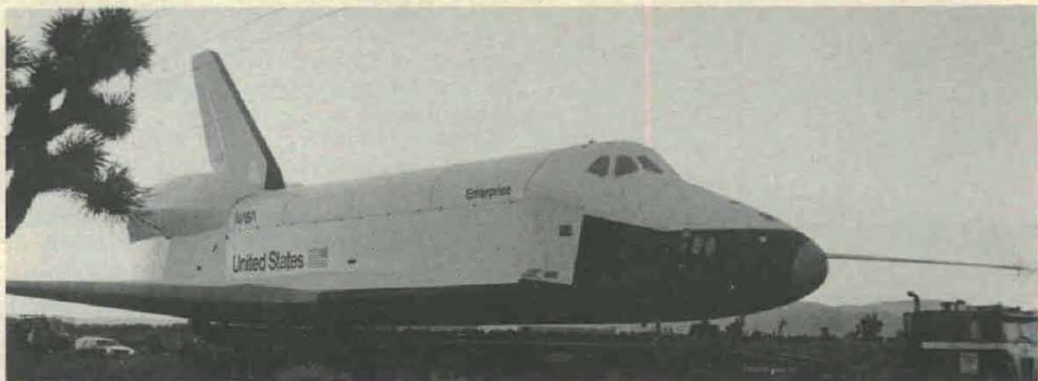
"ENTERPRISE," America's first space shuttle craft, has been mounted atop a Boeing 747 at Edwards Air Force Base, CA, where it is undergoing airstrip taxi tests, prior to "captive" flight tests. The 122-foot-long, 100-ton Enterprise, which has a wingspan of 78 feet and a 60-foot-high tail, is scheduled to be fired into space by disposable rockets in March 1979 from Kennedy Space Center, Cape Canaveral, FL, then return to earth without power and land like a glider. (Photo by Rockwell International.)
