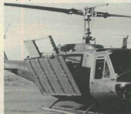
HELICOPTER-MOUNTED antenna, which uses a metal reradiation radar (METRRA) to detect surface mines, is undergoing tests.
