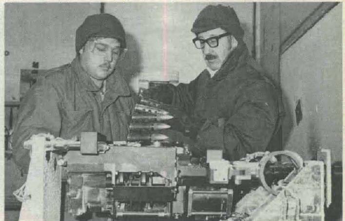
XM230 subjected to extreme cold conditions during DAT.
