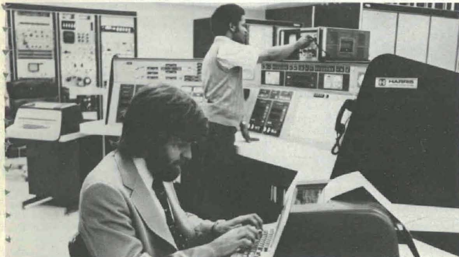
TRANSLATOR operates modified KSR-37 teletype, redesigned to use the Cyrillic alphabet, while a technician monitors two DCL antennas at DCL earth station, Fort Detrick, MD.
