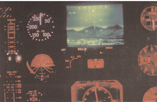
Flight simulator showing Forward-Looking Infrared Radar (FLIR) image from Target Acquisition Designation System (TADS).
