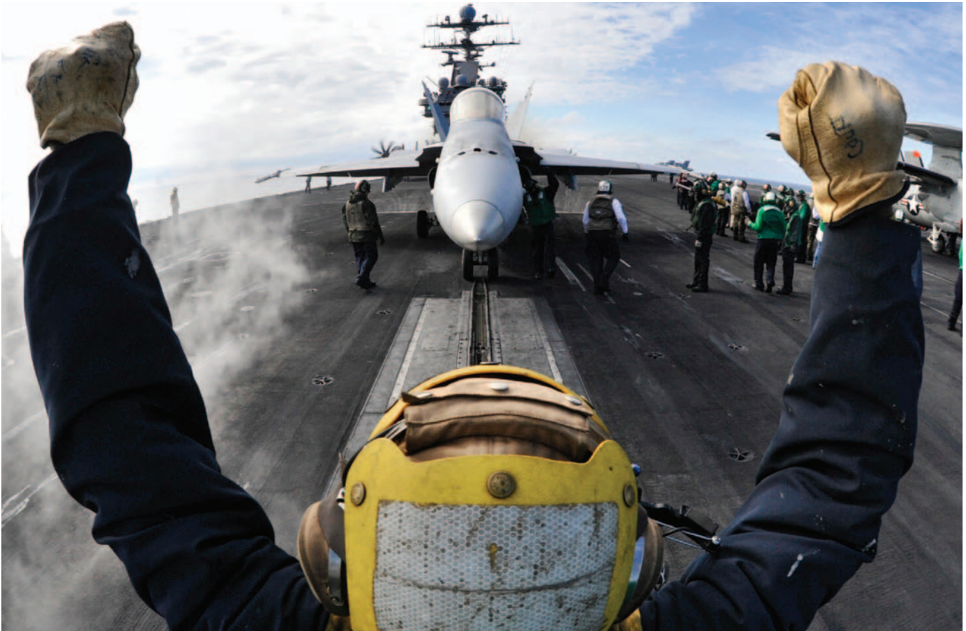
Aircraft director guides F/A-18C Hornet onto catapult aboard USS Harry S. Truman
