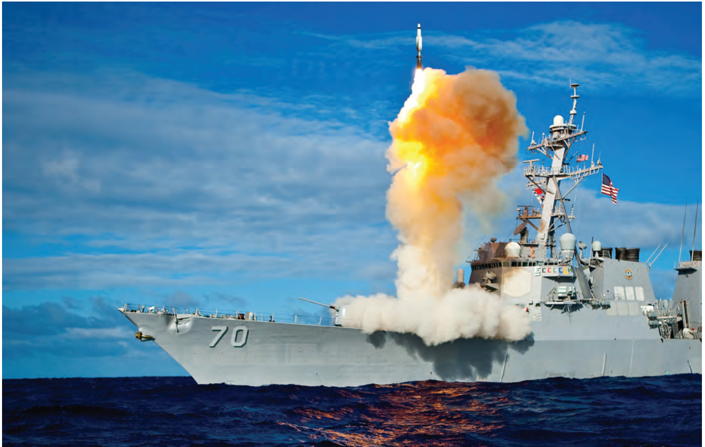
Arleigh Burke -class guided missile destroyer USS Hopper (DDG 70), equipped with Aegis integrated weapons system, launches RIM-161 Standard Missile
