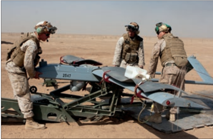
Marines load RQ-7B Shadow UAV onto launching ramp, Camp Leatherneck, Helmand Province (U.S. Marine Corps/Robert R. Carrasco)
