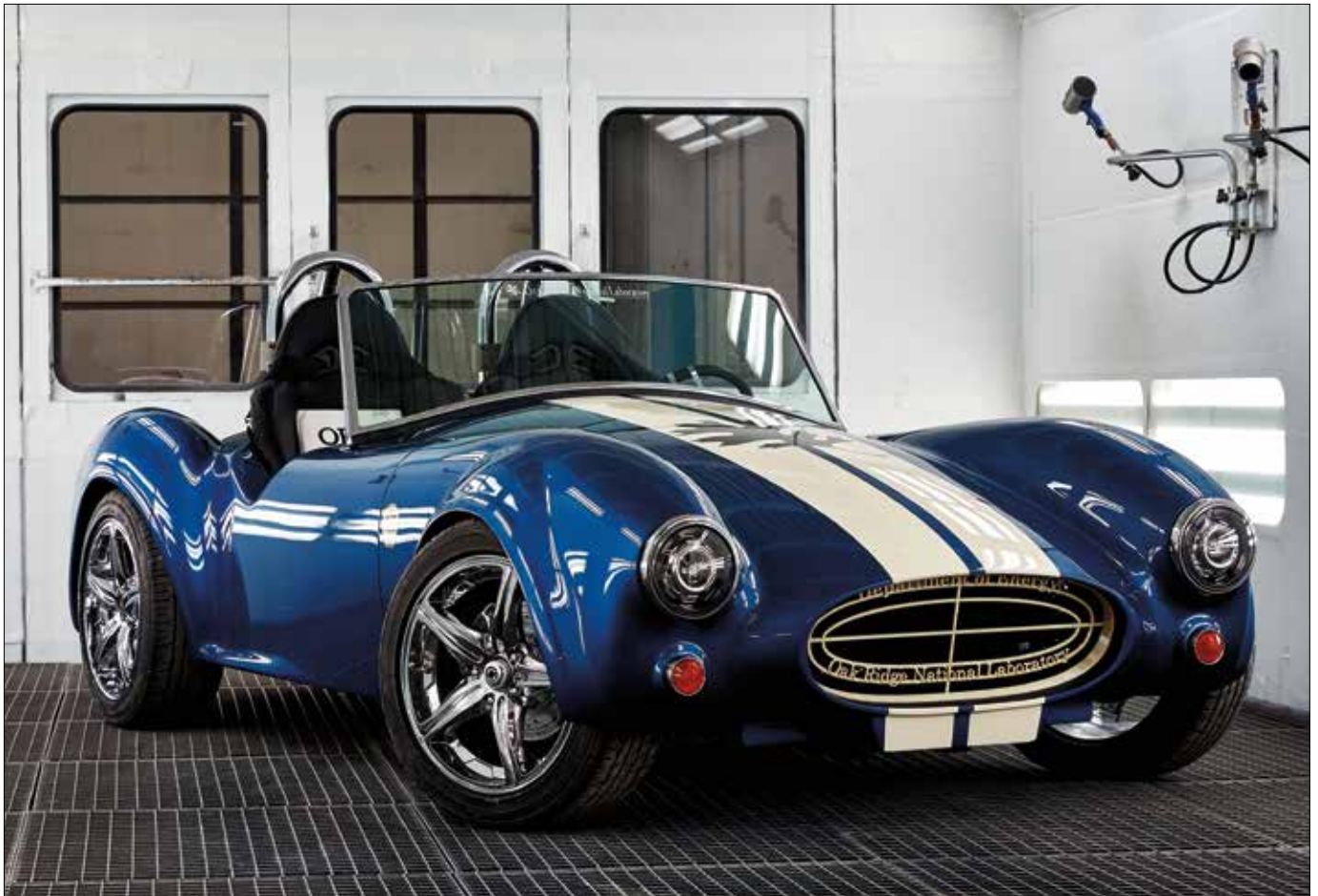
Shelby Cobra—approximately 1,400-pound vehicle containing 500 pounds of printed parts made of 20 percent carbon fiber—produced by Big Area Additive Manufacturing Machine, which manufactures strong, lightweight composite parts in sizes greater than 1 cubic meter (DOE)
