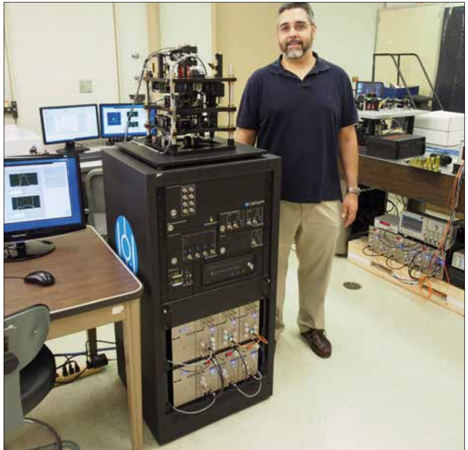
Air Force Research Laboratory Directed Energy Directorate researcher and leader of joint AFRL and University of Hawaii Manoa quantum computing group received two new tabletop quantum computing systems to trap and study behavior of atoms in their condensed, pristine state (U.S. Air Force)
