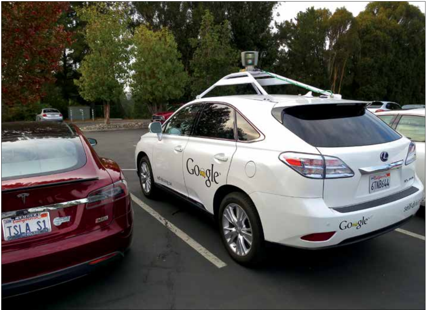
Lexus RX450h retrofitted by Google for its driverless car fleet parked near Tesla Model S electric car (Steve Jurvetson)
