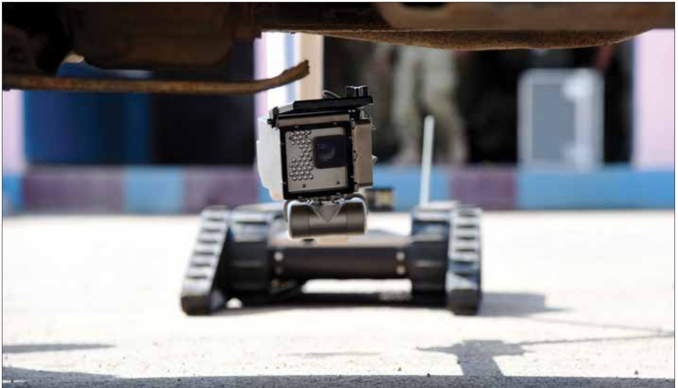
iRobot 510 PackBot searches for explosive devices under vehicle in Djibouti (U.S. Air Force/Maria Bowman)
