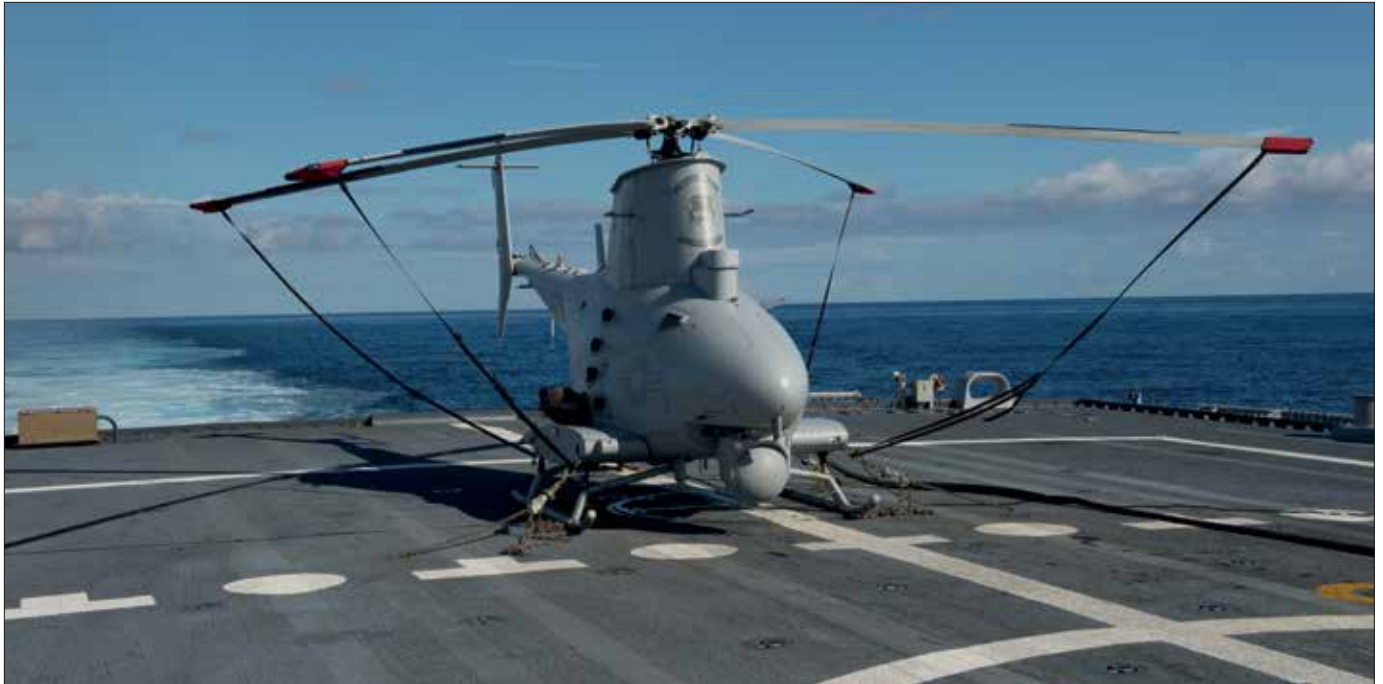
MQ-8B Fire Scout unmanned aircraft system from “Magicians” of Helicopter Maritime Strike Squadron 35 prepares for flight operations aboard littoral combat ship USS Fort Worth (U.S. Navy/Antonio P. Turretto Ramos)
