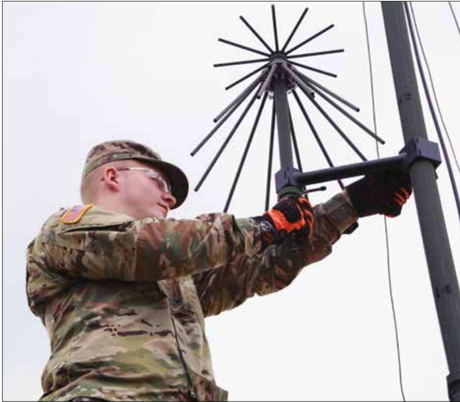
Airman with 38 th Air Defense Artillery Brigade assembles omnidirectional line-of-sight antenna to enable communication with aviation assets during unilateral joint training exercise on Sagami General Depot, Sagamihara, Japan, September 17, 2019 (U.S. Army/Raquel Villalona)
