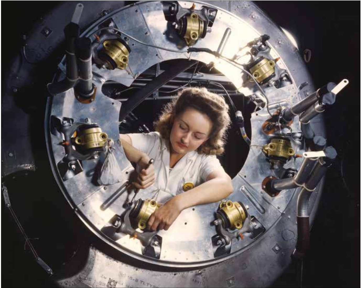
Part of cowling for B-25 bomber motor is assembled in engine department of North American Aviation's plant in Inglewood, California, October 1942 (Library of Congress/Alfred T. Palmer)
