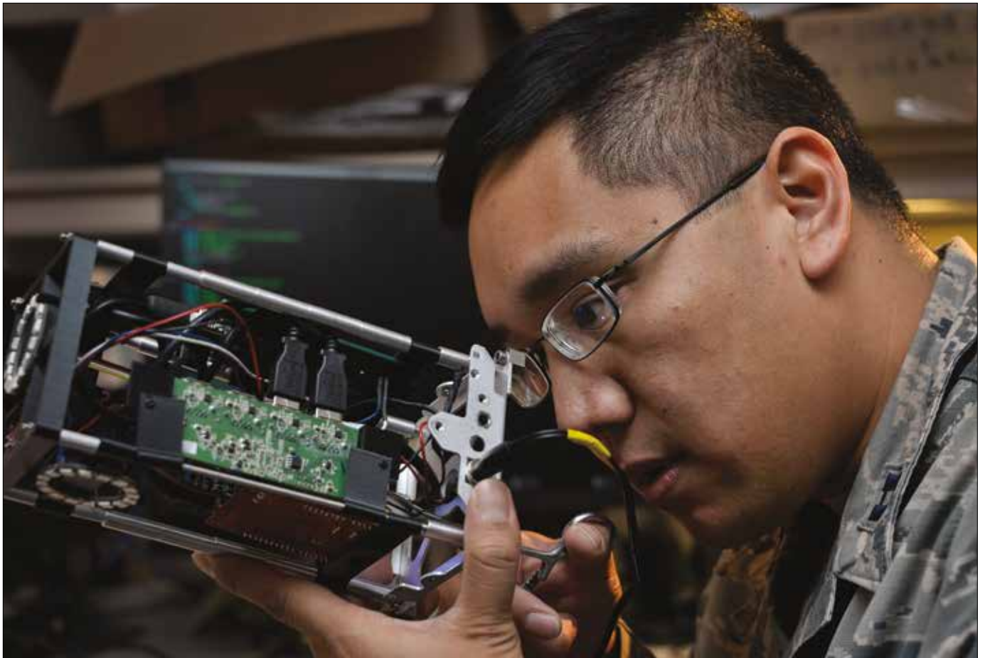
Airman with 707 th Communications Squadron Special Missions Flight repairs connection on CubeSat, in Laurel, Maryland, January 2018 (U.S. Air Force/Alexandre Montes)
