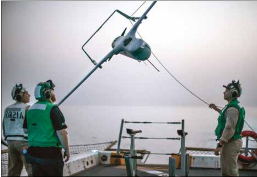
Marines lower RQ-21A BlackJack unmanned aerial system from recovery system aboard USS John P. Murtha , Gulf of Aden, July 2019 (U.S. Marine Corps/Adam Dublinske)
