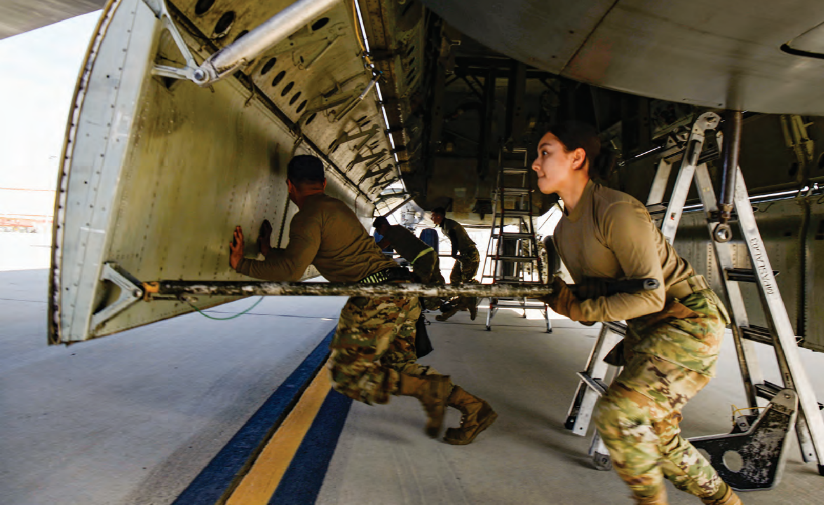
Airmen with 5 th Aircraft Maintenance Squadron push open B-52H Stratofortress bomb bay door to load weapons, December 7, 2021, at Edwards Air Force Base, California (U.S. Air Force/Michael A. Richmond)
