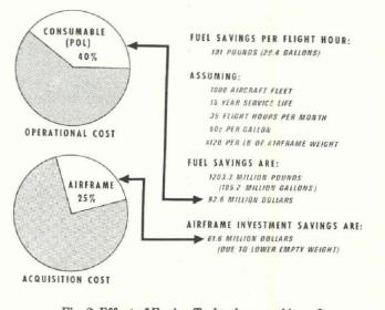
Fig. 2. Effect of Engine Technology on Aircraft (From engine weight and fuel savings only)
