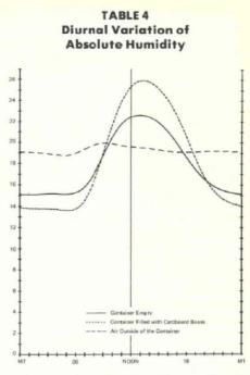
an increase in water-absorbing cardboard. At night the excess water is reabsorbed, preventing significant amounts of internal condensation.
