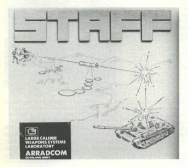
The U.S. Army Armament Research and Development Command, Dover, NJ, has reported "steady progress" in development of a new direct fire antitank weapon system termed the Smart Target-Activated Fire and Forget (STAFF).
