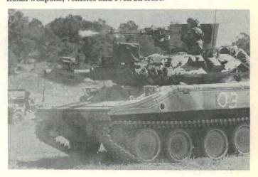
M551 Sheridan equipped with MILES training system. The main gun has the capability of firing one of three lasers to simulate the Shillelagh missile, 152 main gun and coaxial machinegun. Additionally, the cupola-mounted 50-caliber machinegun has its own laser transmitter capability.
