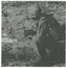
TYPICAL HAND-EMPLACED sensor, with all codes set, is planted in a hole where it will be covered by grass and leaves, leaving only the antenna exposed.
