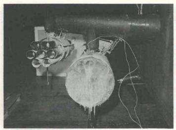
ICE BUILDUP on 2.75-inch rocket launcher, during the month of July, in Alabama, to the required thickness for tests conducted by the U.S. Army Aircraft Development Test Activity at Cairns Army Airfield near Fort Rucker, AL.
