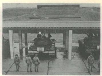
Fig. 2. Tanks on Rocking Platforms on Subcaliber Range.
