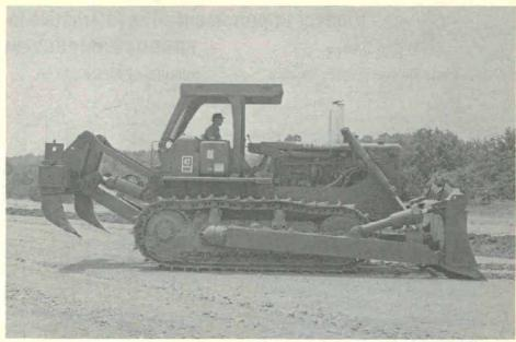
D8K diesel tractor with bulldozer and ripper.
