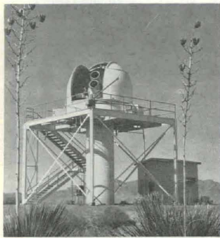
The Distant Object Attitude Measurement System is a twin-barreled tracking telescope used to obtain attitude, event and miss-distance data on missile tests. The system consists of two 24-inch aperture telescopes of 100- and 200-inch focal lengths and high speed 70 mm cameras.
