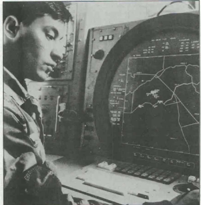
A soldier working at the master computer station plotting PLRS users in the field.
