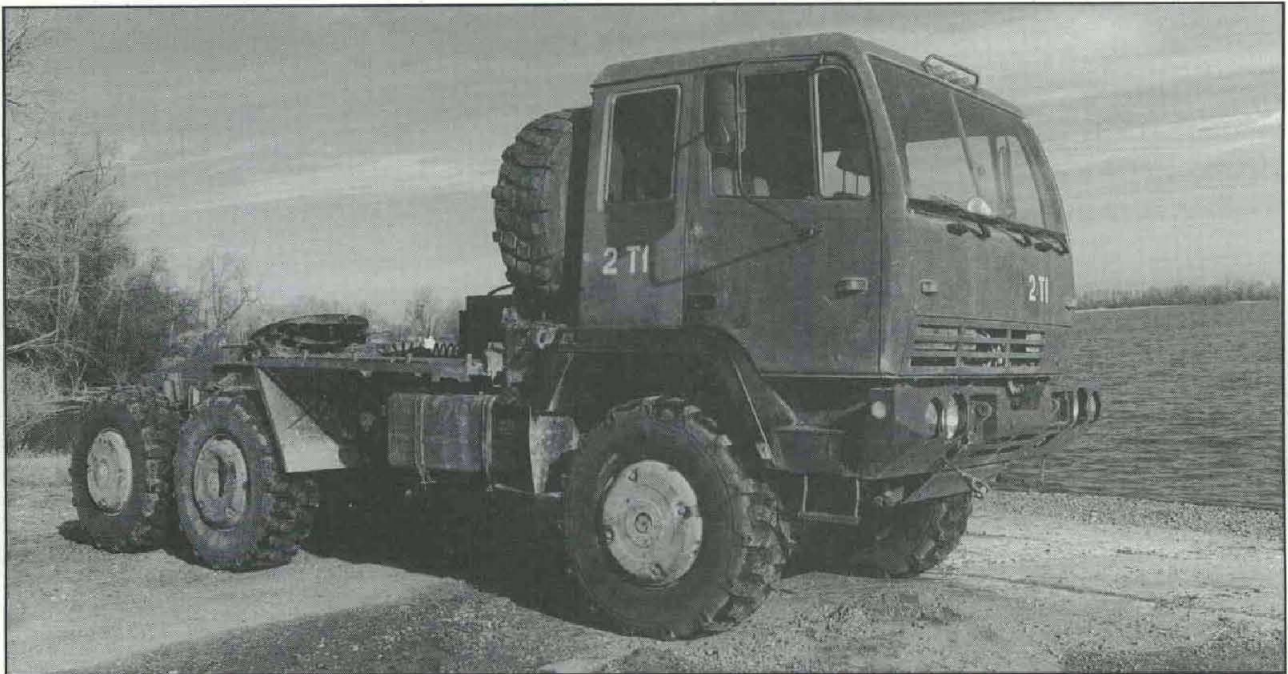
Five-ton tractor version of the Family of Medium Tactical Vehicles.
