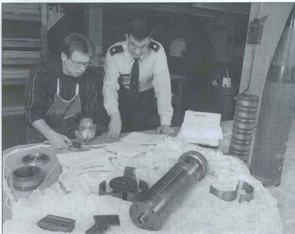
MAJ Charles Dean and West Point's machinist Jeff Butler examine prototype components for the resupply canister that Butler fabricated.
