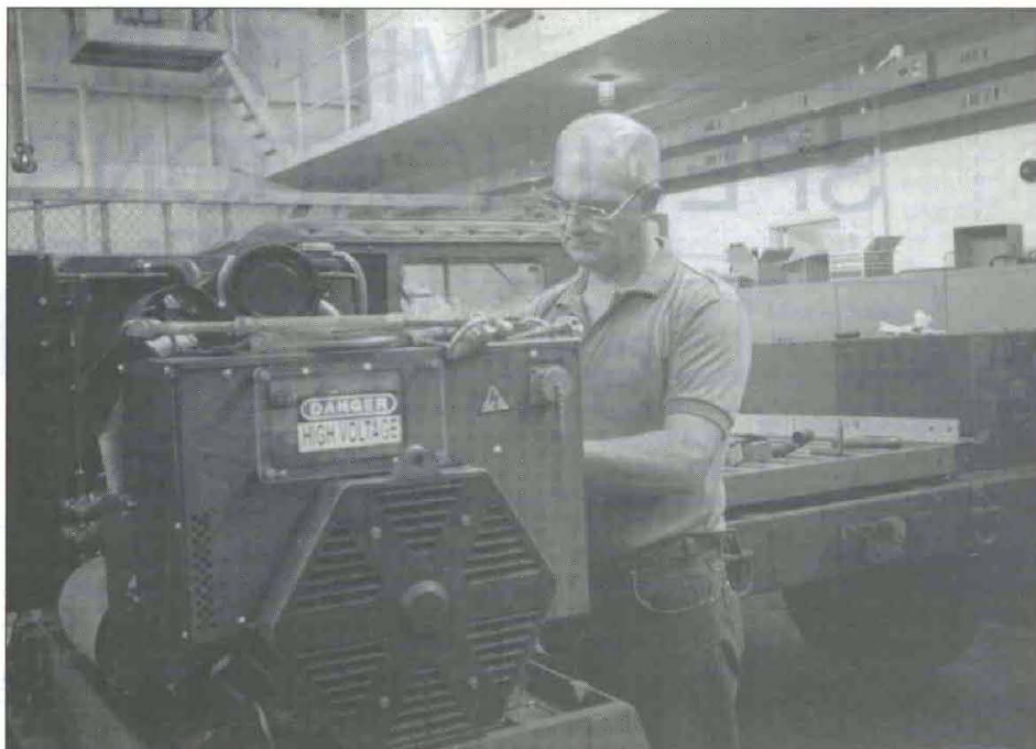
Wayne Shockley, a technician in the Prototype Engineering Division, modifies the crew and cargo storage compartment and mounts a generator on the back of a HMMWV vehicle, prime mover of the GBS Radar.
