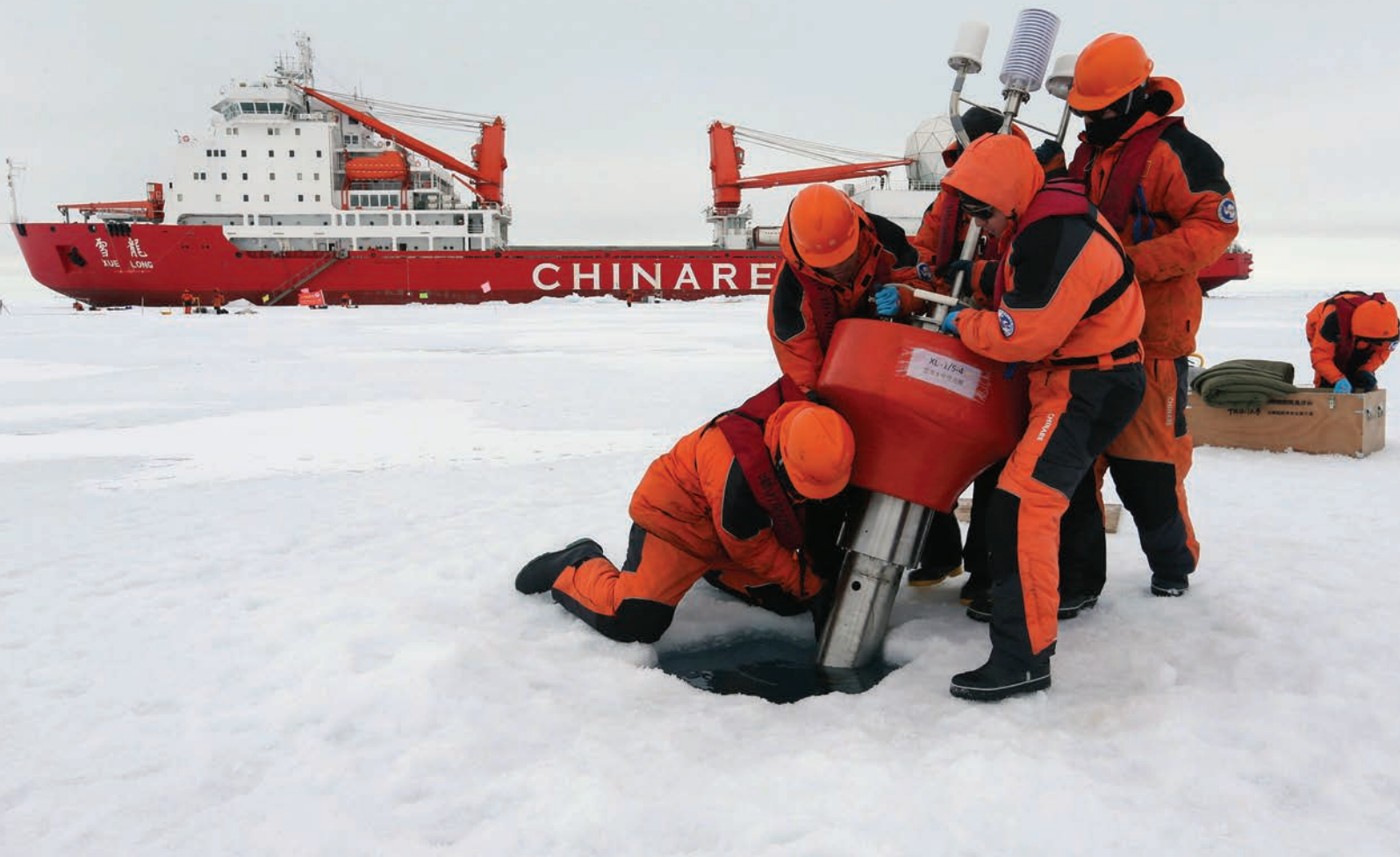
Members of China's research team set up ocean profiling float at short-term data acquisition location near icebreaker Xuelong , or "Snow Dragon," in Arctic Ocean, August 18, 2016 (Xinhua/Alamy Live News/Wu Yue)
